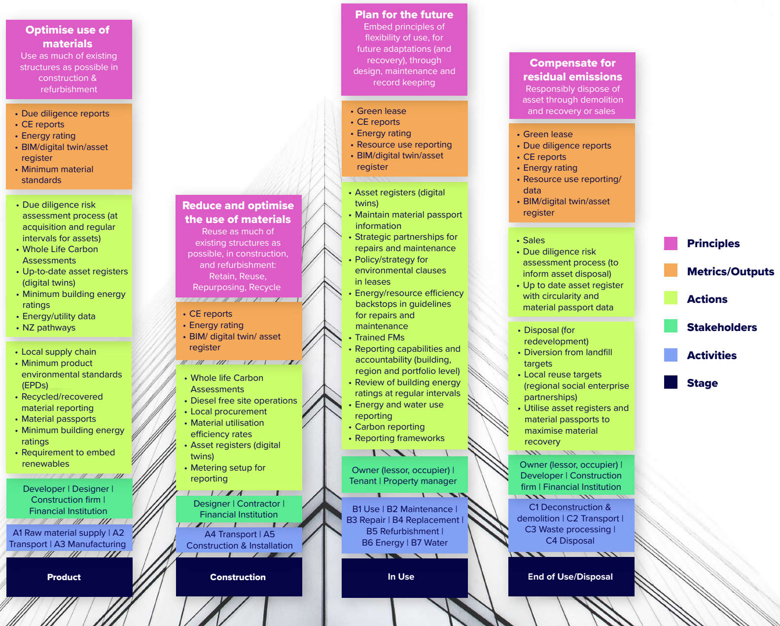
Figure 1: An overview of key actions, metrics and stakeholders across the property life cycle for investors to address whole life carbon emissions
